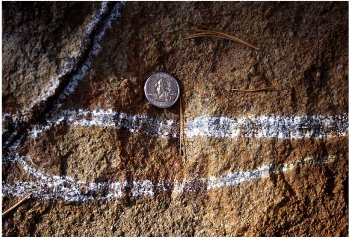
Figure 3. Veins of serpentinite in ultramafic rock from the Emigrant Gap area. Small bands of chrysotile are present within the veins.
